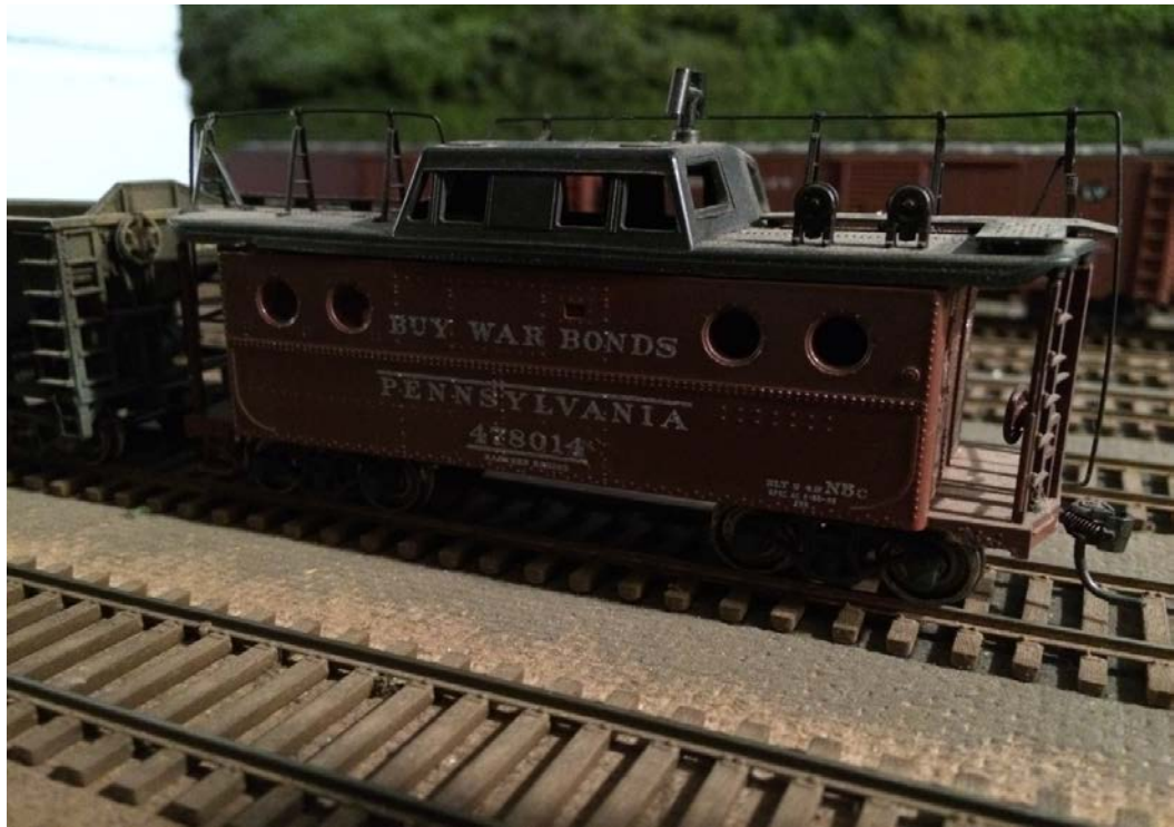
PRR N5C caboose with the period train phone antennas in place.
